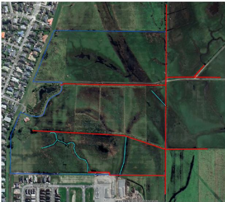
Picture J: Location of main drains (red), some internal shallow surface drains (light blue).
