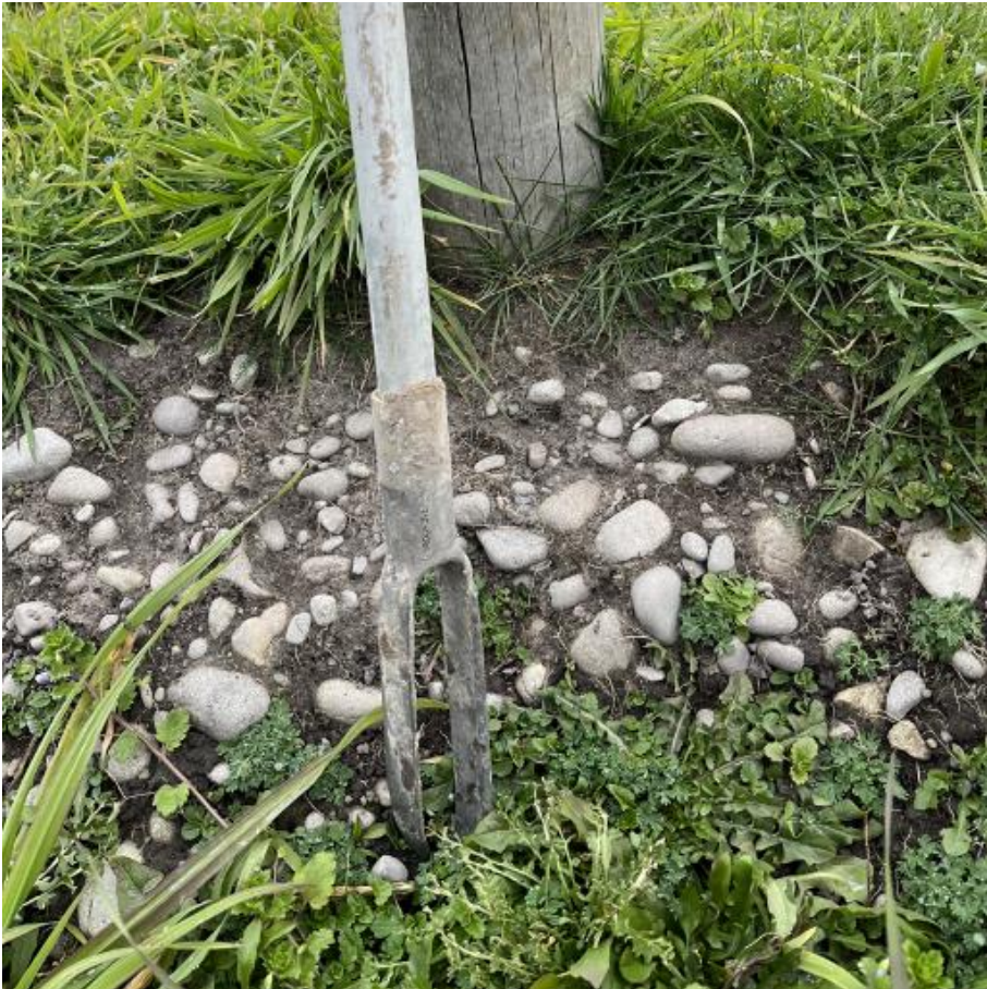
Figure 10: An exposed fence line found at the property shows the gravel content at the surface which stops the auger from being able to be driven into the soil i.e., LUC Class 4s (correlated to 4s7)
