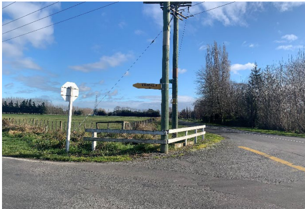
Figure 6: Bradley Road (northbound) intervisibility sight line to left impeded by large utility poles
