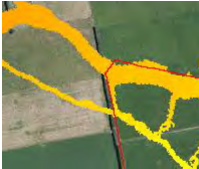
Figure 8 - Pre-development 200yr Flooding
