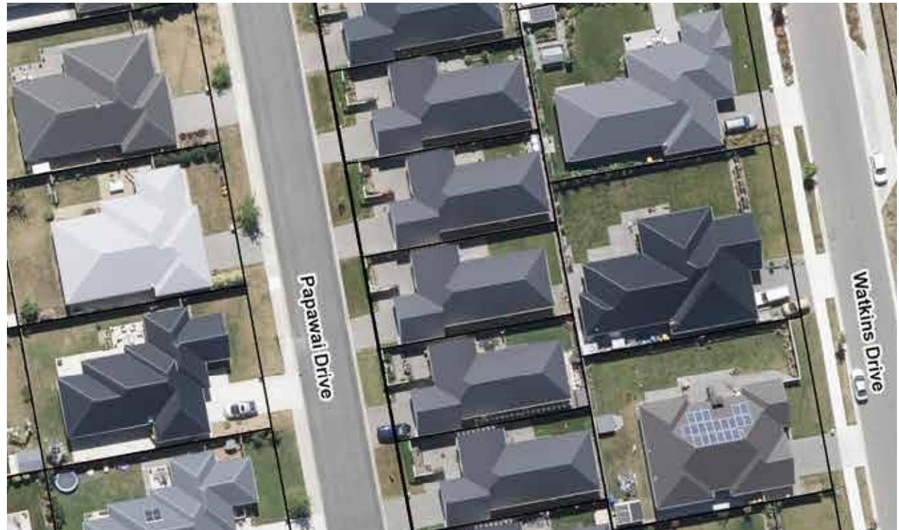
Example : Moderate to high building coverage in Residential 2 Zone, Papawai Drive, Rangiora as a result of dispensations agreed in global consent process resulting in minimal outdoor living space and on site landscaping due to large building footprints.
