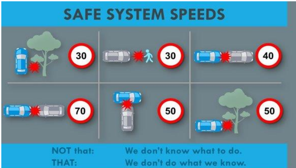
Figure 2. Survivable speeds for different crash type ( Global Road Safety Facility, 2023 ).
