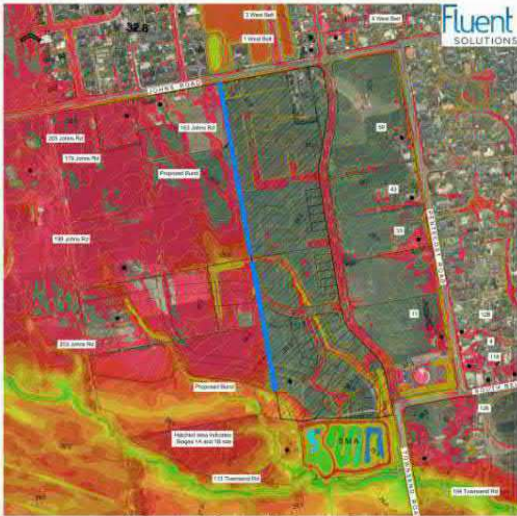
Post Stage 1A and 1B Development Surface and Flood Depth Plan 50 mm Flood Depth Contour Interval
